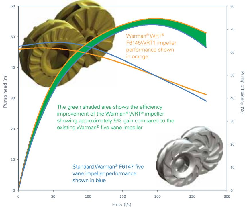
\*Compared to the standard Warman® AH® pump impeller and throatbush combination
